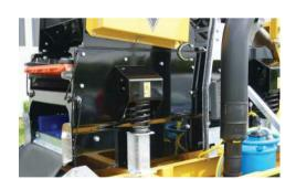
**CONTINUOUS PERFORMANCE.** The heavyweight shaker deck delivers stable performance under variable processing volume. A high capacity 15 hp (11 kW) pump is used for optimum circulation.
