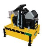
**AVAILABLE AS SKID OR TRAILER.** The R500 reclaimer is available as skid or trailer. The skid is prepared for forklift use, and the trailer comes equipped with a height-adjustable surge brake to adapt to a variety of towing vehicles.
