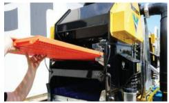
**QUICK-CHANGE SCREENS.** The primary screens are kept in place with an air-clamping system, powered by an onboard air compressor. This allows for ease of access and the ability to quickly change the screens.
