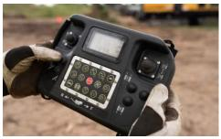
FULL-FUNCTION REMOTE. Adjust machine functions, capture machine data and diagnose equipment fault codes - all from the full-function remote. You can spend more time in the cab throughout the day, monitor machine health and make real-time adjustments remotely, allowing you to keep things running efficiently.
