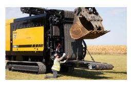
SERVICEABLE BELLY CONVEYOR. The belly conveyor can be removed without detaching the discharge conveyor - allowing for minimally invasive service.
