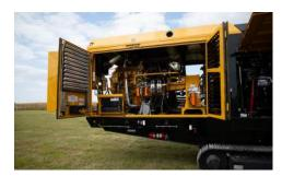
ENGINE BAY ACCESS. The LS3600TX gives you unparalleled access into the machine. The maintenance-friendly and highly accessible engine bay design includes large access doors, multiple ladder points, and a large service platform to help with ease of maintenance and serviceability.
