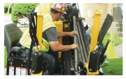
**MULTIPLE ROD OPTIONS.** Equip your drill with either a 6' (1.8 m) 1.66" or 1.31" (4.2 cm or 3.3 cm) Firestick<sup>®</sup> drill rod and save time on the job with 180' (54.9 m) of on-machine rod carrying capacity.
