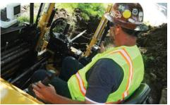
**LOW SOUND LEVELS.** Low noise emission levels at the operator's ear of 85 dBa and a guaranteed sound power of 104 dBa make this drill perfect for installing small utilizes in an urban environment with minimal disruption.
