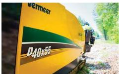
PREMIUM PERFORMANCE. With 40,000 lb (177.9 kN) of thrust/pullback and 5500 ft-lb (7457 Nm) of rotational torque, the D40x55 S3 offers a 10% increase in thrust and rotation over its predecessor, the D36x50 Series II — helping to maximize productivity.
