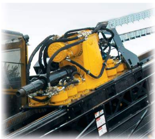
50,000 ft/lbs of torque High torque for drilling in difficult ground formations and turning large back reamers.
