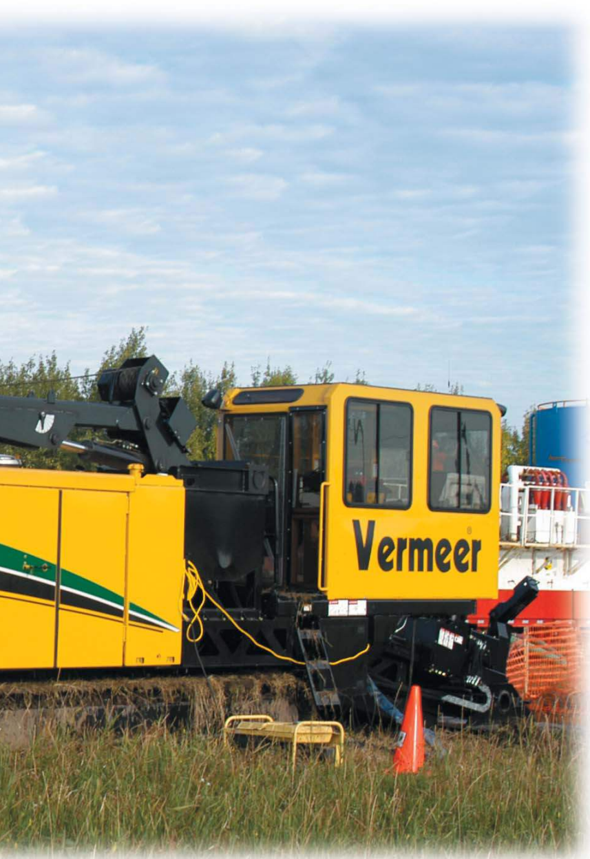
50,000 ft/lbs of torque High torque for drilling in difficult ground formations and turning large back reamers.
