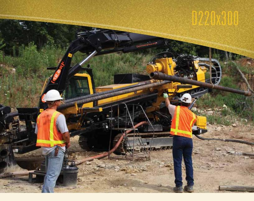
THE VERMEER D220x300 NAVIGATOR® HORIZONTAL DIRECTIONAL DRILL HAS THE POWER OF A MAXI RIG IN A SELF-CONTAINED DESIGN WITH AN ONBOARD DRILLER'S CABIN, MUD PUMP, CRANE AND BUILT-IN ROD STAGER.
