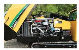
IMPRESSIVE POWER. Powered by a 140 hp (104 kW) John Deere diesel engine, this drill serves up 40,000 lb (177.9 kN) of thrust/pullback and 5,500 ft-lb (7,457 Nm) of rotational torque.
