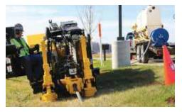
**NEED FOR SPEED.** With a carriage speed of 206 ft/min (62.8 m/min) and a rotational speed of 219 rpm, the D23x30 S3 helps contractors install more linear feet per day, maximizing jobsite productivity and efficiency.
