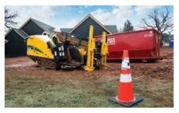
MAXIMIZE PRODUCTIVITY. With 24,000 lb (106.8 kN) of thrust/pullback and 3000 ft-lb (4067.5 Nm) of rotational torque, the D23x30 S3 offers a sizeable increase in power over its predecessor, the D20x22 Series II — helping to maximize machine and jobsite productivity.
