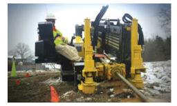
**COMPACT CONTROL.** A width of 55.5" (141 cm) makes the D23x30DR S3 drill 24.5" (62.2 cm) narrower than its closest competitor, offering efficient maneuverability of the machine into compact urban areas or busy neighborhoods, and convenient transportation on a trailer with other equipment.
