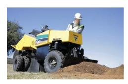
**OPTIONAL HYDRAULIC PUSH BLADE.** The optional hydraulic push blade on the SC382 simplifies jobsite cleanup by helping maneuver processed material.
