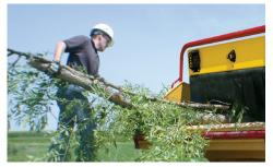
**SMARTFEED.** The patented SmartFeed system helps increase operator productivity while reducing strain on vital engine parts. The feedsensing control system monitors engine rpm and automatically stops and reverses the feed roller when feeding larger, hardwood material.
