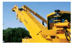
**OPTIONAL LOADING CONVEYOR.** An optional stowable loading conveyor stores easily, and unlike competitive models does not require removal for transportation.
