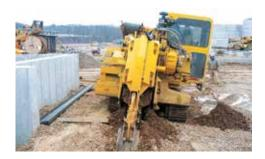
HORIZONTAL SLIDING CAB. A large pressurized/air filtered cab slides 24" (61 cm) horizontally to allow greater visibility for the operator.
