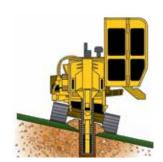
**OPTIONAL AUTO TILT TRACK.** An oscillating track frame allows the track to follow the ground's contour providing a vertical trench on slopes up to 10 degrees.
