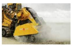
**TERRAIN LEVELER® SURFACE EXCAVATION MACHINE ATTACHMENT.** The T1155III has a chain drive Terrain Leveler attachment option for large rock excavation applications including surface mining, overburden removal, site preparation and road demolition.
