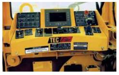
**TEC® PLUS ELECTRONIC CONTROL SYSTEM.** The operating system communicates with multiple control modules located throughout the machine for real-time performance data and advanced troubleshooting capabilities.
