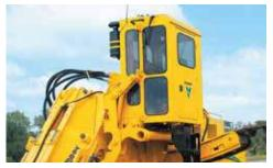
**ELEVATING ROPM CAB.** The spacious elevating rollover protective module cab features LEXAN<sup>®</sup> glass, filtered and pressurized air, heating and air-conditioning. The cab's vantage point allows a virtually unrestricted view of the boom, trench and conveyor.
