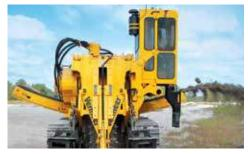
**SECTIONALIZED BRIDGE OPTIONS.** Complimentary to the sectionalized booms, the sectionalized bridge can be adjusted to accommodate a variety of digging depths.
