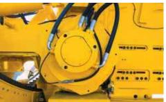
**ROTARY POWER TRENCHER DRIVE MOTOR.** A rotary power trencher drive motor and splined headshaft produce a lower speed and higher torque which provide superior ground penetration and low chain wear for better production results.
