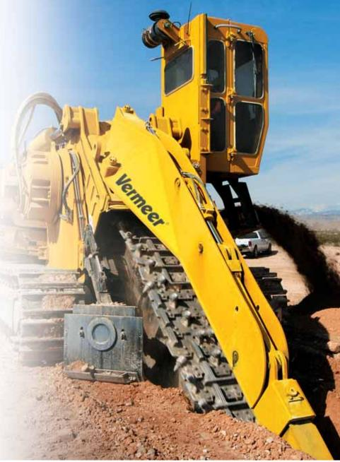
**Sectionalized boom lengths** increase work efficiency. The 6', 8', 10', 12' or 14' (1.8 m, 2.4 m, 3 m, 3.7 m or 4.3 m) boom lengths offer job flexibility and eliminate the time and effort of changing booms.
