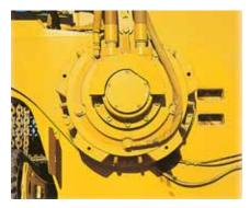
A Rotary Power headshaft and splined headshaft produce lower speed and higher torque, providing superior rock penetration and low chain wear for better production results.
