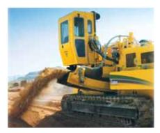
A 415 hp (309.5 kW) Caterpillar Tier 3 engine provides the raw power needed to triumph over tough rock-trenching projects. The engine is emissionized and features high torque rise, allowing engine rpm to recover rapidly in situations that demand increased power.
