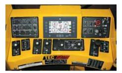
**The new TEC Plus electronic control system** features CAN bus technology, which utilizes multiple control modules located throughout the machine for real-time performance data and advanced troubleshooting capabilities.
