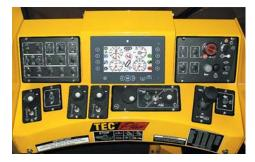
**The new TEC® Plus electronic control system** features CAN bus technology, which utilizes multiple control modules located throughout the machine for real-time performance data and advanced troubleshooting capabilities.
