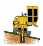
**OPTIONAL AUTO TILT TRACK.** An oscillating track frame allows the track to follow the ground's contour providing a vertical trench on slopes up to 10 degrees.
