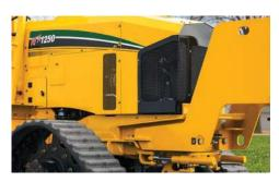
INCREASED POWER. When the RTX1250 engine drops from 2500 rpm to 2300 rpm under load, the horsepower increases from 120 hp (89 kW) to 127 hp (95 kW), allowing the ride-on tractor to run at maximum horsepower in work mode.
