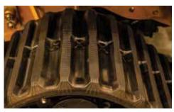
QUAD TRACK SYSTEM. The quad track system offers improved flotation, reduced surface damage, increased tractive effort and greater stability. Four-wheel steer and crab steering are functional with both quad track and tire options.
