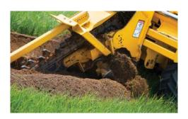
MAKE SENSE OF YOUR TRENCH. When difficult conditions are encountered while trenching causing a sudden drop in engine speed, the TrenchSense<sup>™</sup> feature automatically pauses the forward motion of the tractor to prevent engine shutdown and recalibration of the machine controls. Once pre-set engine and trencher speed recovers, forward AutoCreep resumes. The sequence occurs within seconds and requires no operator adjustment.
