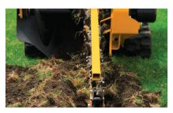
**OUTBOARD BEARING SUPPORT:** This feature provides protection for the headshaft when trenching in difficult conditions, helping to lower the overall cost of operation.
