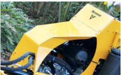
MINIMIZE SERVICE TIME AND TOOLS. You know serviceability isn't an option. The engine cover design offers virtually "no-tool" access to all daily and weekly service points, making for quick service turnaround.
