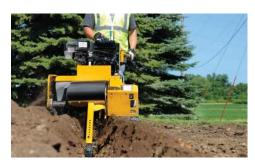
SLENDER PROFILE. A 35" (88.9 cm) width allows the RTX130 to access small spaces including passing through typical backyard gates.
