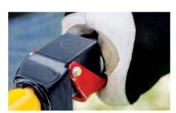
**OPERATOR PRESENCE SYSTEM.** Promotes on-the-job safety that disengages the trencher and ground drives if the operator leaves the controls, in addition to a trenching cleat that restricts backward motion.
