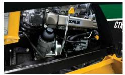
**OPTIMAL POWER.** Equipped with a 40-hp (30 kW) turbocharged Kohler KDI diesel engine. This engine meets emission compliance without the need for a diesel particulate filter (DPF), reducing cost and complexity of the engine.
