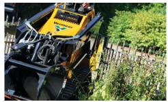
PRODUCTIVITY. Maximum tipping capacity of 2958 lb (1341.7 kg) and a rated operating capacity of 1035 lb (469.5 kg) for efficient lifting in tough ground conditions.
