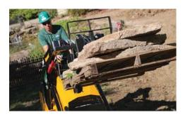
ADAPT TO THE CHALLENGE. The option of a wide 9" (22.9 cm) track or a narrow 7" (17.8 cm) track and a universal mounting plate allows you to work with a variety of attachments on the job.
