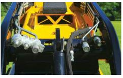
**HYDRAULIC BOOST.** The S925TX comes standard with a dual hydraulic auxiliary system with high flow to power the most demanding attachments and a low flow to give the operator maximum control.
