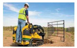
A DEDICATED SPRING-CUSHIONED PLATFORM keeps the operator out of the mud. The integrated operator presence system suspends ground drive and powered boom/bucket motion when the operator steps off the platform.
