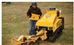
CHOOSE YOUR VIEW. The side operator's station offers the ability to select the best angle from which to view the stump during operation and provides all control functions for cutter wheel and ground drive creep forward and reverse.
