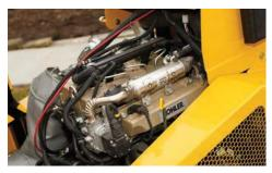
POWER AT THE STUMP. A 40 hp (29.8 kW) T4 Final diesel engine provides substantial power and uses a DOC after-treatment system, which offers reduced maintenance and could lower operating costs.
