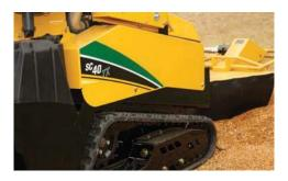
**ALL TERRAIN.** A counter-rotating track undercarriage enhances maneuverability by making it easier to reposition when cutting a stump. The tracks also offer good floatation and the ability to operate in less-than-ideal ground conditions.
