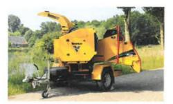
**CONVENIENT 180° SLEW RING.** Allows the chipper infeed to be rotated to face the material for ease of feeding and convenience when working along the roadside.
