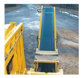
**Continuous undermill conveyor system.** Designed to handle large volumes, the 36" (91 cm) wide conveyor belt has a maximum speed of 640 fpm (195 m/min) and a height capability of 14" (4.3 m).
