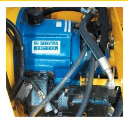
**Optional PT Tech clutch.** Push-button engagement reduces the chance of operator error, and allows the operator to engage the clutch via remote, cab, or ground control station. Clutch engagement is maintained by oil pressure, eliminating the need for clutch adjustment and also provides torque limiting protection. What's more, the clutch is backed by a 1-year/1,000-hour limited warranty.
