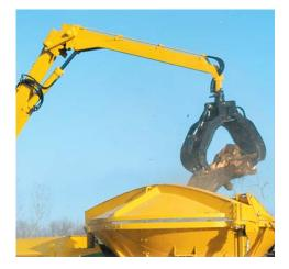
**Optional loader.** With a 27' (8.2 m) reach and continuous rotation multi-tine grapple, the loader has the ability to lift up to 3,500 lbs (1,588 kg) at full reach.
