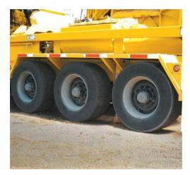
**Ground clearance.** A tandem or triple axle suspension with super single tires provides flotation and 11" (28 cm) of ground clearance for better transport and movement in areas where soil conditions are unstable. The enhanced clearance also provides protection of components under the machine, such as brake canisters and axle components, by keeping them up and out of the way of debris that is commonly found on jobsites.
