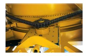
Hydraulic tub drive chain tensioner. A hydraulic cylinder increases tension on the drive chain when the tub rotation circuit is under load, reducing periodic adjustments. Continuous tub chain sprocket provides positive drive at any load.
