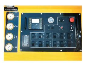
**Control panel.** The control panel display of the microprocessor and CAT engine systems, provides real time performance data. The control panel also provides full instrumentation and diagnostic gauges for monitoring hydraulic systems and troubleshooting. The panel is located under the Falling Object Canopy, which helps protect the operator from falling debris.
