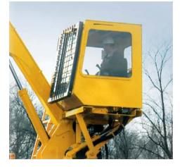
**Ergonomic cab enclosure and cab controls.** The optional loader cab pivots with the loader, allowing greater visibility and reducing operator movement during normal working conditions. Filtered and pressurized incoming air, heater, and air conditioner provide greater operator comfort. Once the machine is started from the ground control station, virtually all operations can be controlled from the cab.
