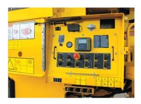
**Control panel.** A centralized control station provides real time performance information and full instrumentation. The control panel is also equipped with diagnostic ports for monitoring systems and troubleshooting.
