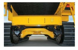
**Ground clearance.** The HG4000TX is designed with 16" (41 cm) of ground clearance, enhancing the unit's ability to traverse difficult terrain.
