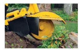
**SMOOTH OPERATION.** The exclusive SmartSweep<sup>™</sup> control system monitors engine load and provides continuous feedback, resulting in a smooth and consistent cutter wheel sweep rate.
