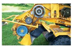
**CONVENIENT BELT SERVICING.** Belts on the SC362 are serviceable from one side of the machine with cutter drive belts being adjustable with movable idlers. Additionally, each belt set may be adjusted independently, without affecting adjustment of other belts.
